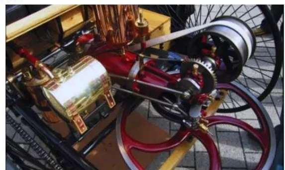
Engine of the first Patent Motorwagen, presumably from the replica
