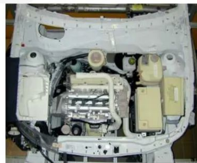
PMU(Physical Mock-Up) of a vehicle engine compartment
