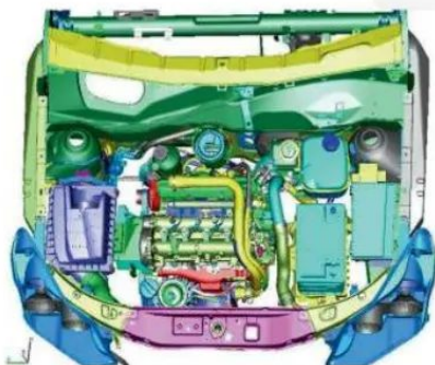
DMU(Digital Mock-Up) of a vehicle engine compartment
