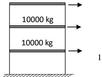
The damping may be assumed as 5% for all modes. Using response spectrum method calculate the base shear.
