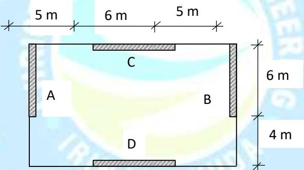
11. A slender shear wall of length 6 m and thickness 200 mm carries an axial load of 2700 kN. The wall is reinforced with 10# bars at 250 mm c/c in two layers. If M25 concrete and Fe415 steel are used, estimate the moment of resistance of the wall.
